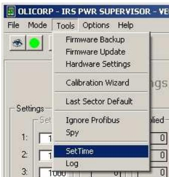
To set up the Real Time Clock (RTC) it is necessary to set up USB connection. You need a USB cable with connector on the IRS side and the SUPERVISOR program. We advise to use USB cable with special filters. If the USB connection is established successfully, the USB LED will light on steadily.
