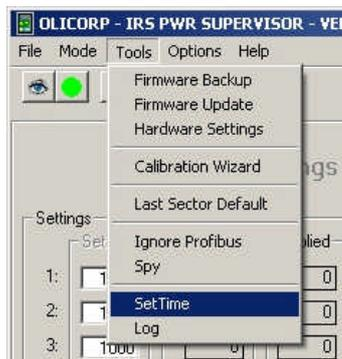
Switch the PC or NoteBook ON. Start up **SuperVisor**. Select the COM port corresponding to the virtual USB COM port. If the USB connection is kept OK, the green LED near the USB connector on the MCU board must be glowing permanently. Next you need to select **SetTime** from the menu. At his moment your PC time will be set for the RTC Datalog, and the window with the current RTC value will open (see pic. below).
