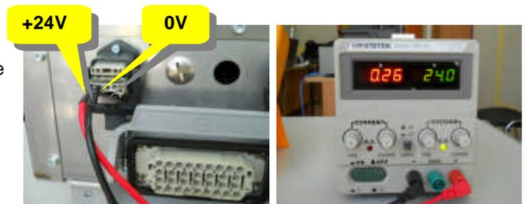
Open the IRS box door and switch the both breakers “close”. Set your Multimeter to resistance measuring mode and select the measuring limit - MOhms. Place one multimeter probe on IRS box, place the other probe at one of the power connector poles (as shown in Fig). Wait for the reading on the Multimeter display to stabilize.
